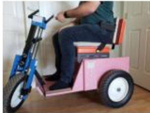
Turning: Rotate wheel in desired direction and spin arm pedals forward or back as desired.
