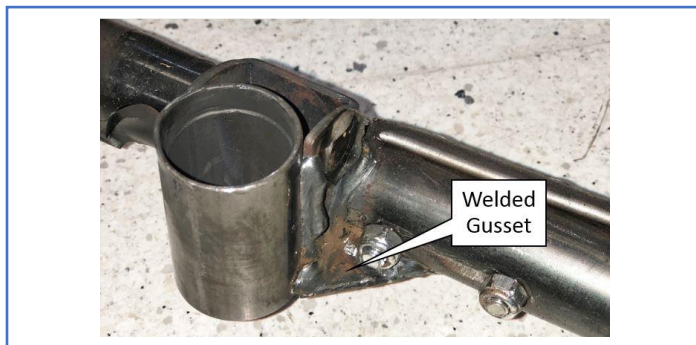
Figure 4. Improved GEN_2 with welded gusset.
